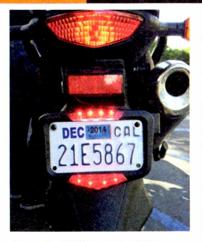
Above: The Vololights flash a brief diagnostic sequence on power-up to ensure functionality. Not only can you see the white LEDs for the license plate, but you can see how bright the red LEDs are compared to the stock brake light. Below: Wiring in the unit was very easy, but we took our time for a very clean and stock-looking final appearance.
